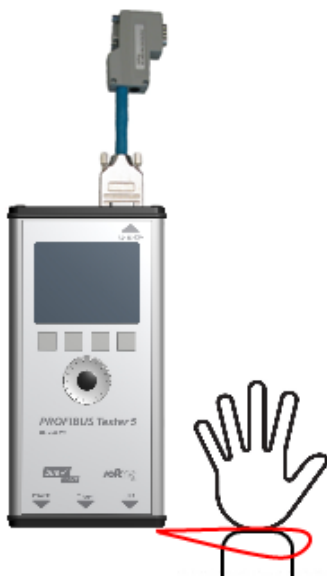
Figure 16: Recommended use of retaining strap
