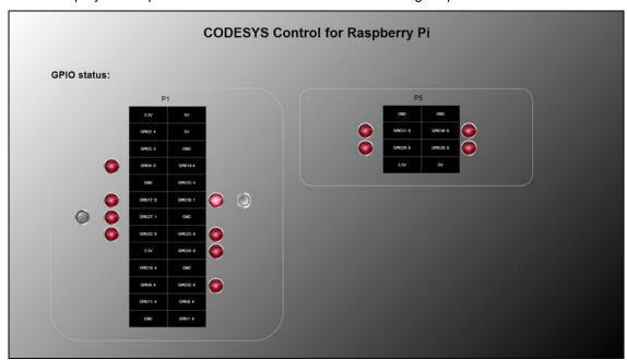
For using the additional GPIOs of the hardware variant Raspberry Pi B+ we provide you with a separate GPIO device, that can be plugged into the slot "GPIOs" in the device tree.
