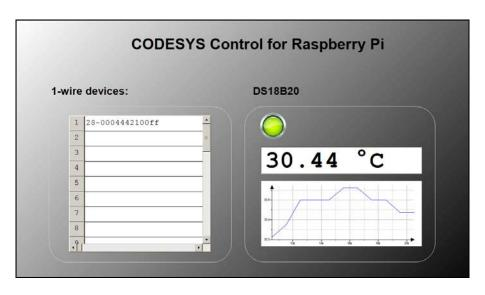
Note that the data exchange via 1-wire takes quite a lot of calculation time in this implementation, during which the task is blocked. Therefore it is recommended for time critical applications to assign the 1-wire devices to a task of low priority (see device configuration, tab I/O exchange, buscycle options).
